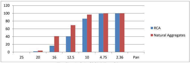
Fig:- Sieve Analysis of RCA & Natural Aggregates
